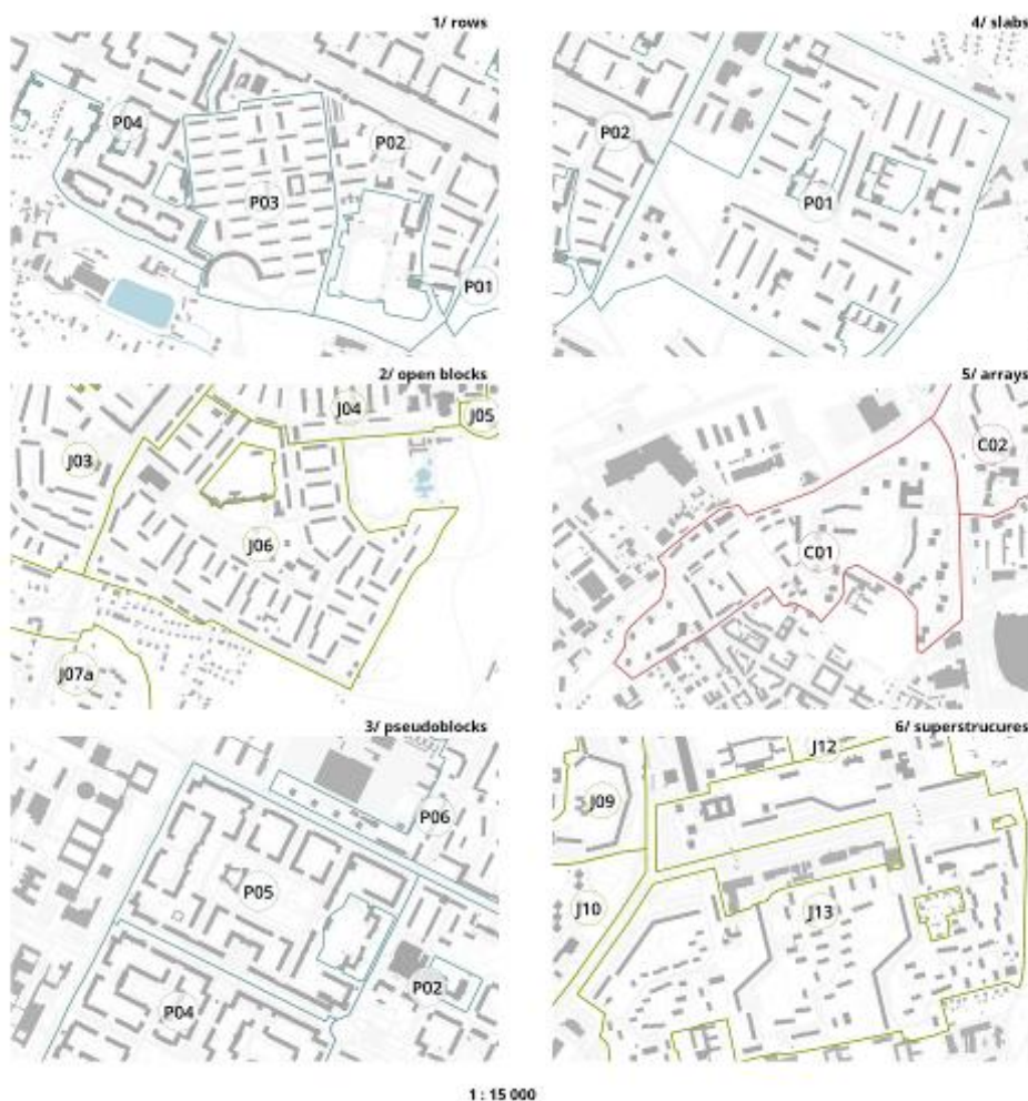
Figure 2: Typology of housing-estates' urban structure.
