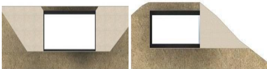
Figure 8: Underground house with a free facade
